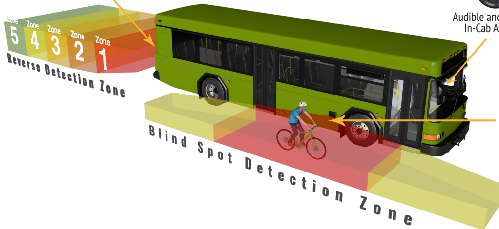
PreView Sentry ® Detection Zone Adjustable from 0 to 30m (98')
