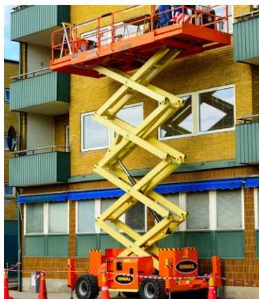
Rough Terrain (engine-powered) scissor lift
