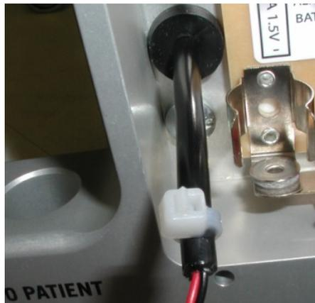
**Step 5.** Cut the wire between the zip tie and the rubber strain relief.
