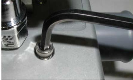
**Step 2.** Using a ball-end of a 5/32" Allen (hex) wrench, remove the top stainless steel set screw holding the flow meter. (The wrench must be held at angle. The screw will not come out of the hole, but the flow meter will come off the front.)
