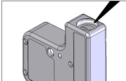
**Step 4.** Position a new fitting in the opening of the hole and insert the fitting into the hole. Strike the part gently with a plastic mallet to ensure the part snaps into place.
