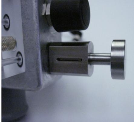
**Step 10.** Place the device on its end and press the orifice into place using an arbor press. The orifice is seated when the positioning tool knob is fully depressed as shown.
