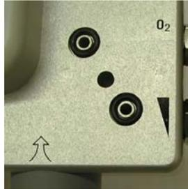
**Step 11.** Carefully line up the body of the device over the flow meter so the grooves for the o-ring line up with the o-rings on the flow meter.
