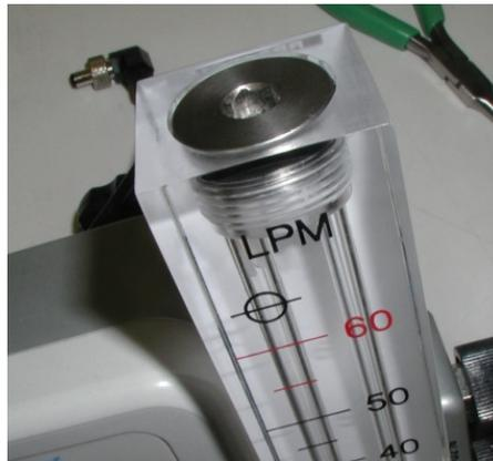
**Step 9.** Check to make sure the ball rolls freely back and forth in the flow meter.
