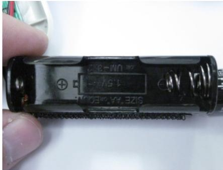
**Step 4.** Reinsert the battery holder on the Velcro strip.
