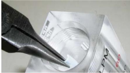
**Step 6.** Tilt the flow meter to remove the ball.
