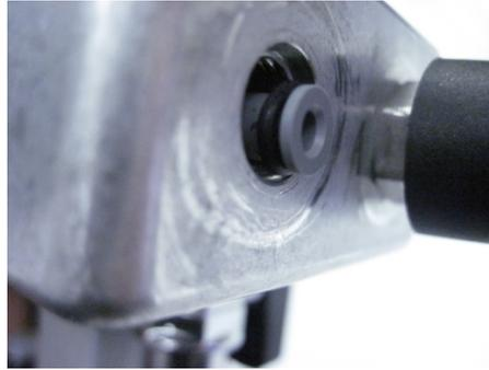
**Step 7a.** Insert the small o-ring (RP56P02-901) onto the outside of the new orifice.
