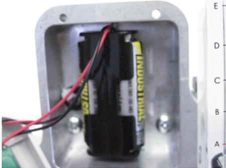
**Step 5.** Connect a sensor to the sensor cable. Turn the unit on and verify that the unit powers up and that a reading shows up on the LCD screen. Verify that the battery symbol is no longer displayed.
