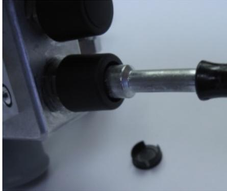
**Step 2.** Use a 1/2" open ended wrench to remove the valve cartridge.
