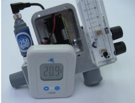
**Step 6.** Align the MaxVenturi Analyzer Assembly to the edges of the main body and reattach it using the 4 screws removed in step 1.
