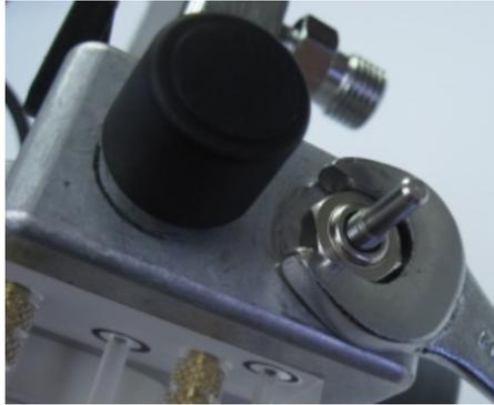
**Step 6.** Repeat the preceding steps to replace the o-rings of the O2% valve cartridge
