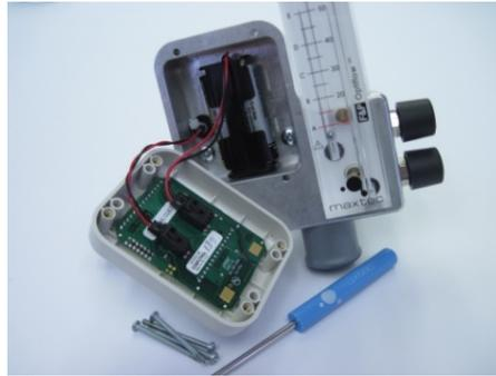
**Step 2.** Disconnect the two wire connections by pressing in the center of the connector and pulling lightly on the wires.
