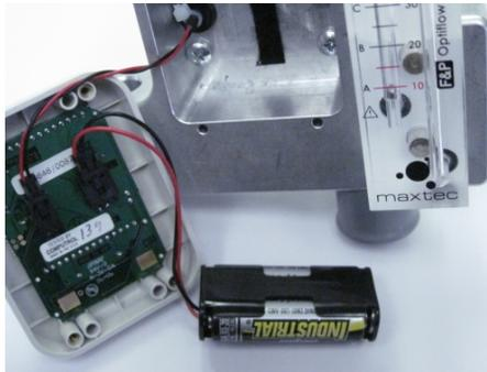
**Step 3.** Insert new batteries. Ensure that they are oriented correctly following the diagram on the battery holder.
