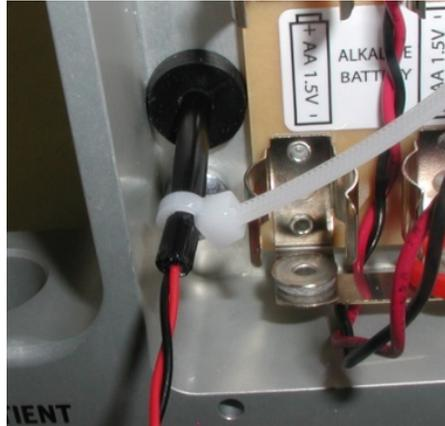
**Step 10.** Clip off the excess length of the zip tie and pull on the cable till the zip tie is against the rubber grommet inside the main cavity.
