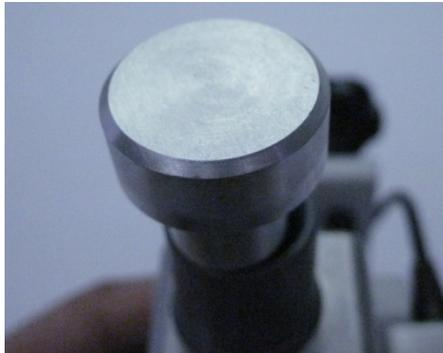
**Step 5.** Use an arbor press to push out the orifice. Apply increasing amounts of force gradually until the part is removed.
