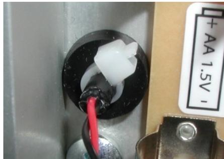
**Step 11.** Apply a few drops of glue on the zip tie next to the cable.
