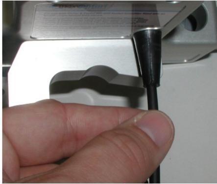
**Step 8.** Remove the replacement cable from its packaging and insert the stripped end of the wires into the rubber strain relief in the back of the unit. Pull on the cable till approximately one inch of the shielded cable protrudes into the main cavity of the unit.
