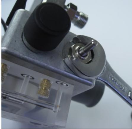
**Step 5.** Reinstall the black knob by placing the knob over the valve stem and tightening the retaining nut with a 7mm nut driver while holding the knob.
