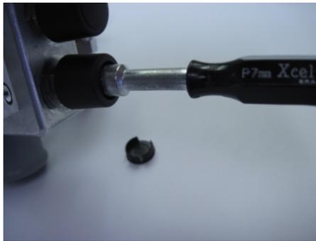
**Step 6.** Install the cap on the new knob. Be sure to align the wide gap in the cap with the two protruding ribs inside the cap.
