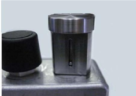
**Step 11.** Remove the orifice insertion tool by twisting the tool counter-clockwise.
