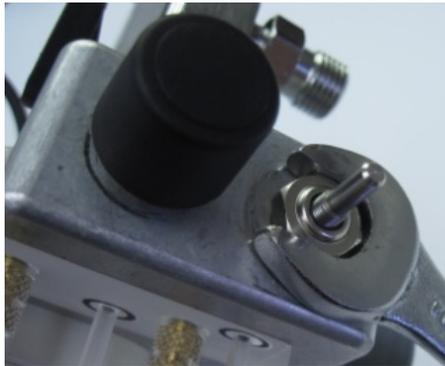
**Step 3.** Remove the two o-rings from the valve cartridge.
