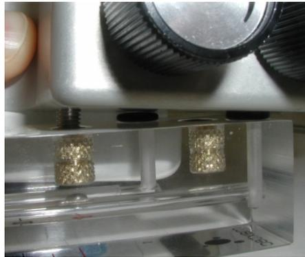
**Step 12.** Fasten the flow meter in place with the two stainless steel screws removed in steps 1 and 2. It works best to start both screws before tightening both of them.
