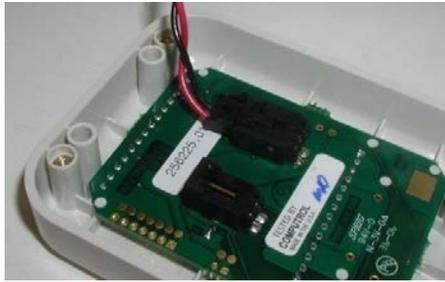
**Step 5.** Attach the sensor cable (smaller connector) to the appropriate connector (small connector) on the PCB of the replacement MaxVenturi Analyzer.
