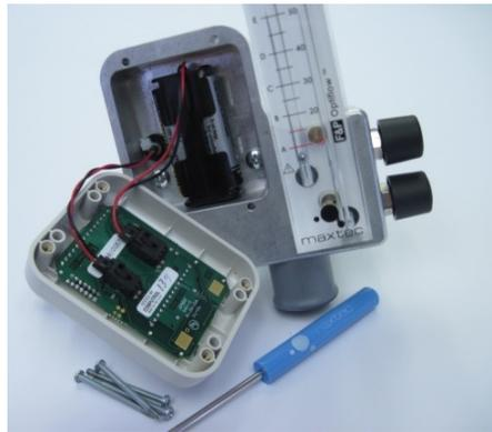
**Step 2.** Detach the two electrical connectors from the back of the printed circuit board (PCB). Push in the center of each connector to open the latch of each connector.
