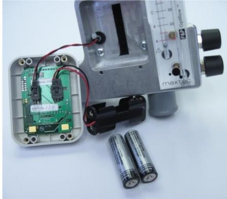
**Step 4.** Push on the cable from the back to break any glue that is sticking to the cable and the rubber strain relief.
