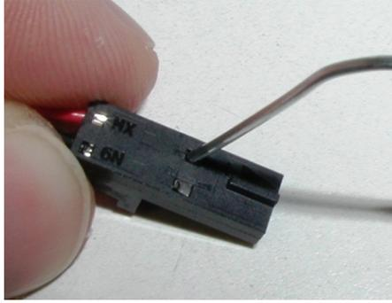
**Step 7.** Carefully pull the wire out from the rubber strain relief through the back of the device.
