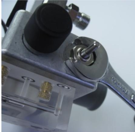
**Step 3.** O<sub>2</sub> control cartridge (R211P30-002 for 0-60 LPM MaxVenturi, or R211P30-004 for 0-120 LPM MaxVenturi) and flow control cartridge (R211P30-001) are different. Check to make sure the replacement cartridge matches the cartridge being replaced.
