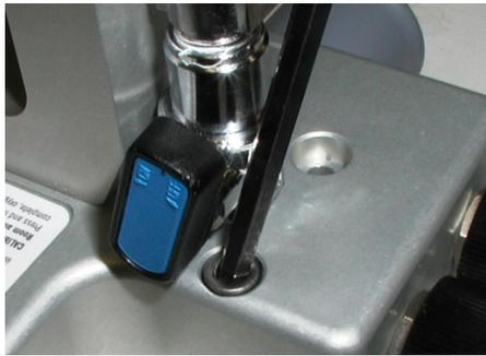
**Step 3.** Two o-rings sit in grooves on the front of the unit. It is suggested that these O-rings be replaced during maintenance. Contact Maxtec Service Department for replacement o-rings.
