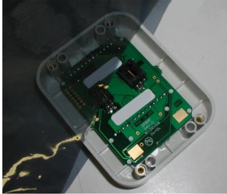
**Step 4.** Attach the battery cable (larger connector) to the appropriate connector (larger connector) on the PCB of the replacement MaxVenturi Analyzer.
