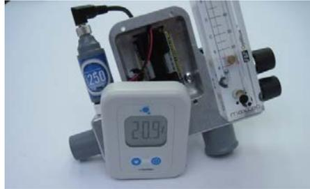
**Step 16.** Align the MaxVenturi Analyzer Assembly to the edges of the main body and reattach it using the 4 screws removed in step 1.
