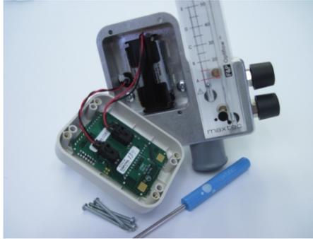
**Step 2.** Take out the battery holder. Remove the dead batteries from the holder. A screwdriver or other tool may be used to pry the batteries out.
