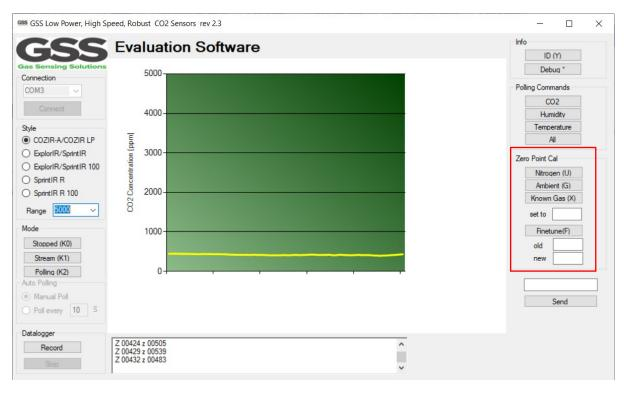
There are a several methods available to the user to set the zero point of the sensor. In all cases, the best zero is obtained when the gas concentration is stable, and the sensor is at a stabilised temperature. Note the zero-point settings are not cumulative and only the latest zero-point setting is effective. For example, there is no benefit in zeroing in nitrogen, and then zeroing in a calibration gas. The sensor will store only the latest zero point.
