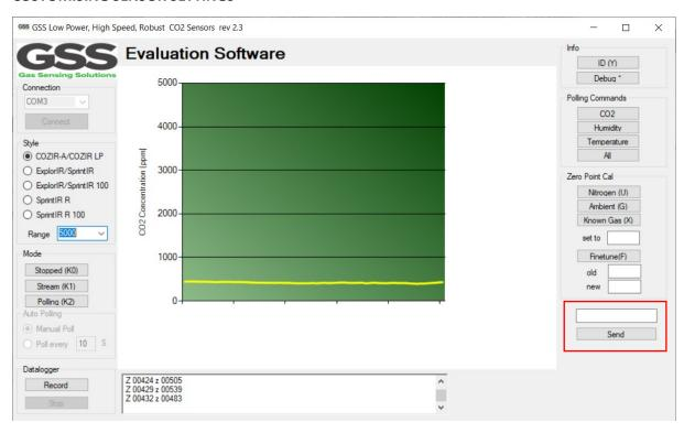
The evaluation kit software allows the user to fully customise the settings of the sensor. Refer to the sensor data sheet for a full command and control description. All UART commands and functions of the sensor can be manually set by writing in the blank box with the correct syntax. To send an UART command or data to the sensor, write in the blank box and click the 'SEND' button.
