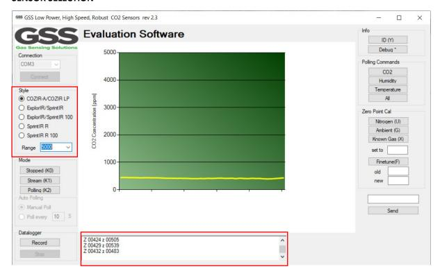
Select the correct sensor type and the full-scale range ( $CO_2$  ppm) of the sensor. The sensor should automatically start to take  $CO_2$  measurements after 1-2 seconds. These measurements are shown graphically in the middle of the screen, and in the dialogue box (red) at the bottom. The dialogue box contains sensor serial data output ('Z' data). The  $CO_2$  'Z' value needs to be scaled to calculate the ppm value.
